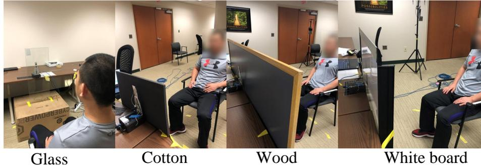
Figure 4.13: Experiment setup with different blockage materials.
