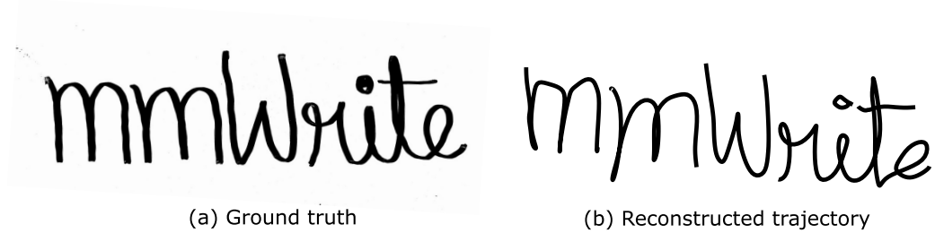
Figure 5.1: Illustration of handwriting tracking using the proposed mmWrite system. (a) Picture of the handwritten trajectory and (b) Reconstructed trajectory of the word “mmWrite”.
